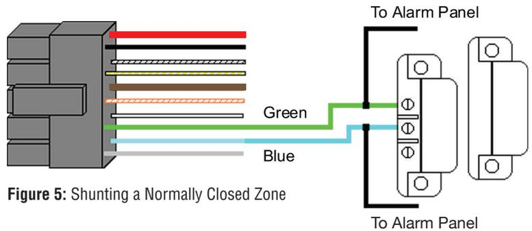
Figure 5: Shunting a Normally Closed Zone
