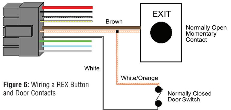
Figure 6: Wiring a REX Button and Door Contacts
