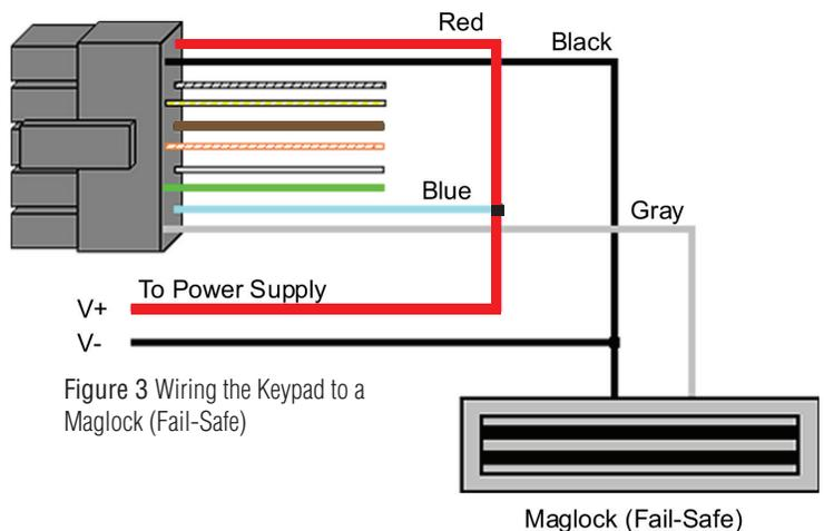
Figure 3 Wiring the Keypad to a Maglock (Fail-Safe)
