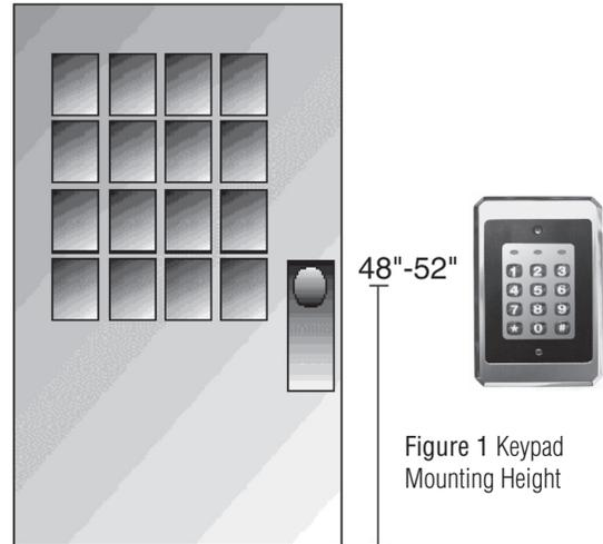
Figure 1 Keypad Mounting Height
